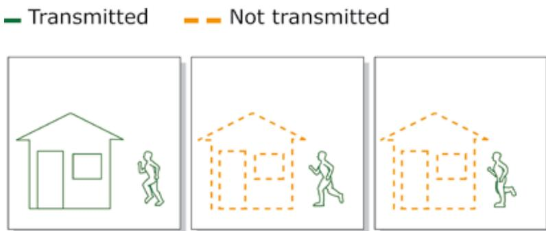
Figure 4. With difference coding (used in most video compression standards including H.264), only the first image (I-frame) is coded in its entirety. In the two following images (P-frames), references are made to the first picture for the static elements, i.e. the house, and only the moving parts, i.e. the running man, is coded using motion vectors, thus reducing the amount of information that is sent and stored.
