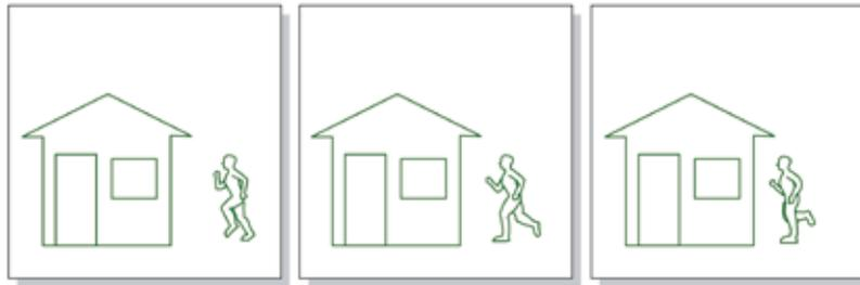
Figure 3. With Motion JPEG format, the three images in the above sequence are coded and sent as separate unique images (I-frames) with no dependencies on each other.
