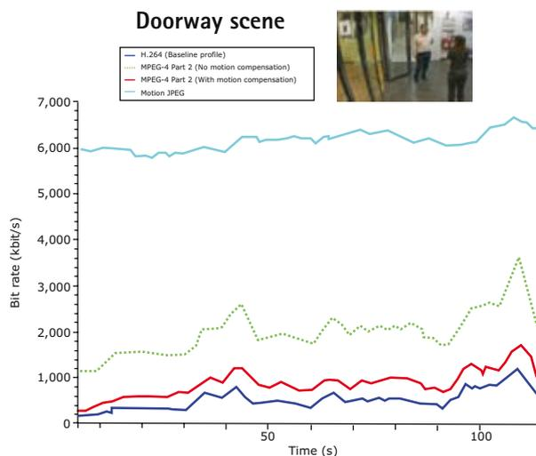
Figure 1. An H.264 encoder generated up to 50% fewer bits per second for a sample video sequence than an MPEG-4 encoder with motion compensation. The H.264 encoder was at least three times more efficient than an MPEG-4 encoder with no motion compensation and at least six times more efficient than Motion JPEG.
