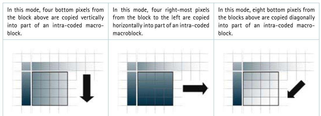
Figure 6. Illustrations of some of the modes that intra prediction can take in coding 4x4 pixels within one of the 16 blocks that make up a macroblock. Each of the 16 blocks in a macroblock may be coded using different modes.
