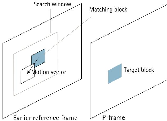
Figure 5. Illustration of block-based motion compensation
