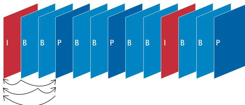
Figure 2. A typical sequence with I-, B- and P-frames. A P-frame may only reference preceding I- or P-frames, while a B-frame may reference both preceding and succeeding I- or P-frames.
